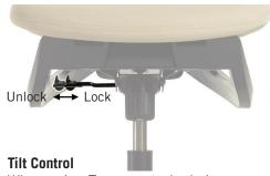
When using Trey as a task chair, you can lock the back into an upright position. Push the tilt control handle in toward the center of the chair to lock. To tilt, return the handle to its extended position.
